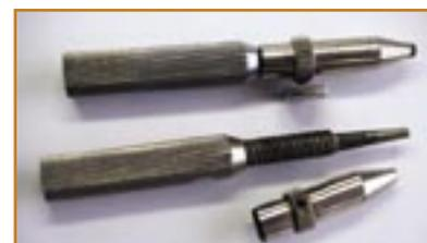
Figure 5. Dr. Okuda's original punches (1.5 and 2mm)
