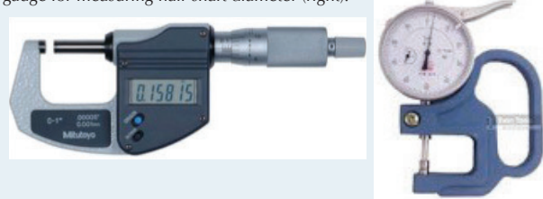
FIGURE 5. Digital micrometer for measuring hair shaft diameter (left); thickness gauge for measuring hair shaft diameter (right).
